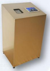
A microphone recognizes the alarm status of the inserted detector and finds out if the alarm was triggered correctly by analyzing the devices audio signal. In this way the test will be concluded as successful or failed. Every successful test will be logged in a database. If the check fails, the user can eventually create a comment by using the software keyboard and quit the test as successful.
